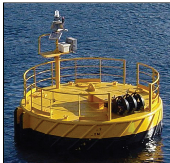
Figure 3. Example off-shore single buoy (Source:Bluewater Shipping BV)
